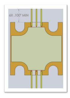
Figure 8. Excess Interconnect Supplied for Next Assembly
