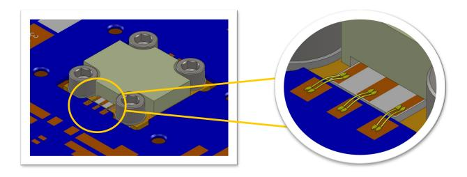
Figure 5. CMPA2560025F MMIC Power Amplifier Wire Bonded at Next Level Assembly
