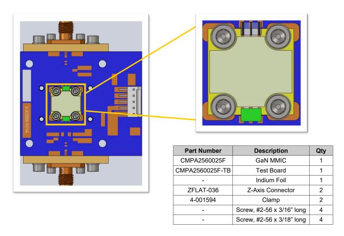
Figure 4. Top View Showing Compression Strip Approximately Centered over Test Fixture and MMIC Amp Traces (Clamps Hidden for Clarity)
