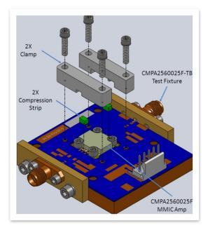
Figure 2. Exploded View of CMPA2560025F MMIC Power Amplifier and CMPA2560025F-TB Test Fixture
