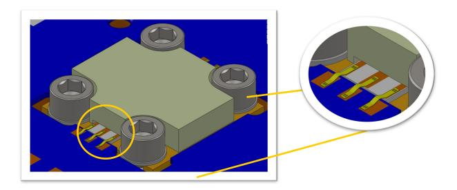
Figure 6. Illustration of CMPA2560025F MMIC Power Amplifier Gap Welded at Next Level Assembly
